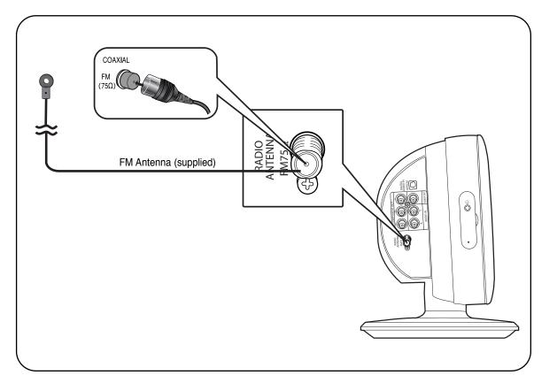
**1** Connect the FM antenna supplied to the FM 75 $\Omega$  COAXIAL terminal.
